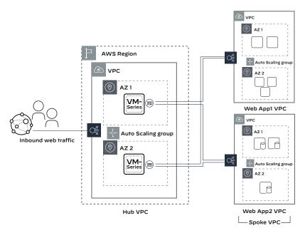
Figure 2: Auto Scaling with the VM-Series on AWS
